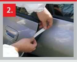
2. Apply tape behind the door edge taking care to place the adhesive behind the panel. Leave the adhesive free portion extending beyond the door edge.
