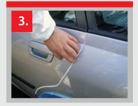
3. Close the door. Adjust the tape into the gap to the required length.
